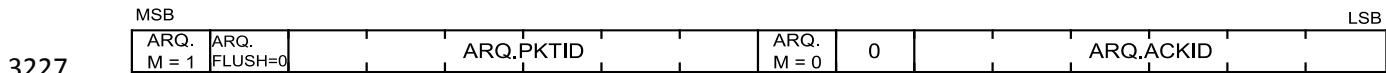
3228 Figure 110 - Stop and wait ARQ subheader without data and with an ACK
